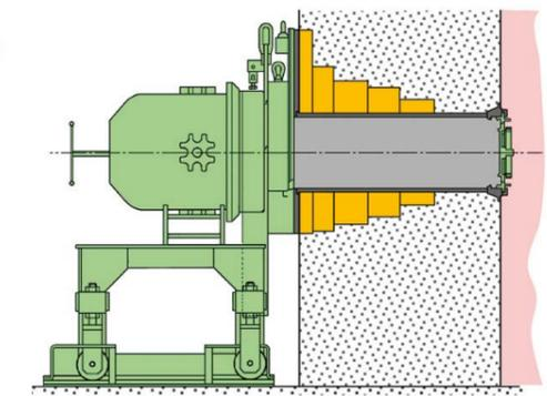
PADIRAC™ docked onto a concrete wall ( DPTE® gamma type mounting)
