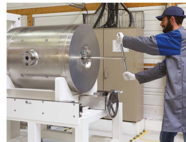
Like the PADIRAC™, the AGNES system offers alpha, beta and gamma protection levels in a single piece of equipment. It contains a cluster holder basket which can be interfaced with a DPTE® 105. AGNES provides operator and environmental security, fast loading and unloading and transport on public roads.
