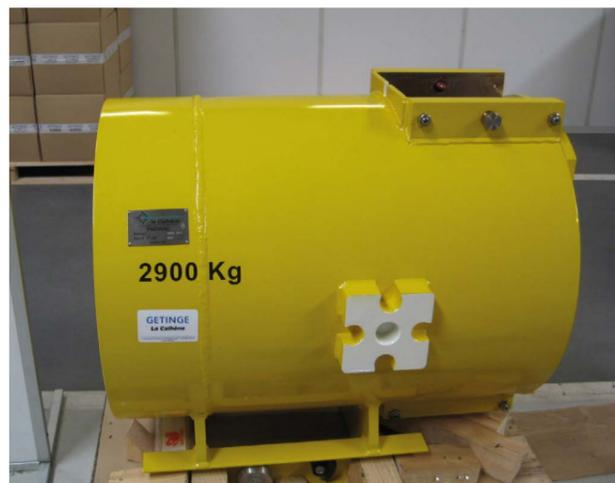
AEB is designed for a DPTE® 105 mm diameter connection. Its shielding can be adapted to requirements (150, 200 and 250 mm thick lead) ; likewise, its length is variable as needed. AEB by La Calhène is primarily used for nuclear medicine applications, for transport inside a facility.
