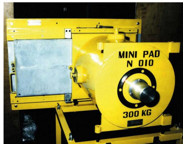
The MINI-PADIRAC, is used for applications similar to those of the PADIRAC™ since it holds the same leaktight container, but its lighter shield (25 mm thick lead) makes it suitable for less radio-active products. Containment during transfers is provided by a DPTE® 270 container. The MINI-PADIRAC is used to extract low activity waste (alpha, beta, gamma), bring a new item inside the cell and/or for transferring equipment between two cells.
